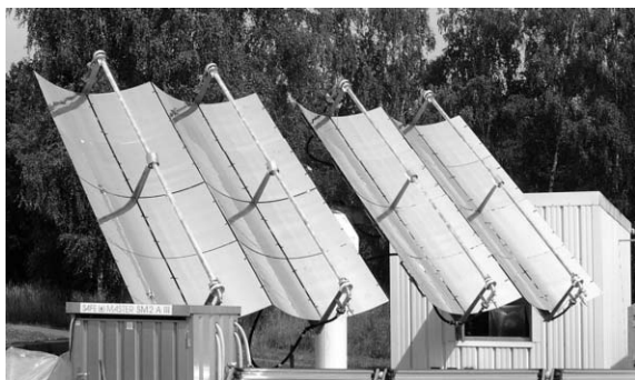
Fig. 1 PROPHIS reactor during the photooxygenation of citronellol 1 .
