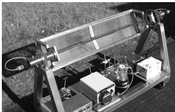
Fig. 4 Small scale parabolic trough reactor equipped with holographic mirrors during the solar photooxygenation of 1,5-dihydroxynaphthalene 3 .
